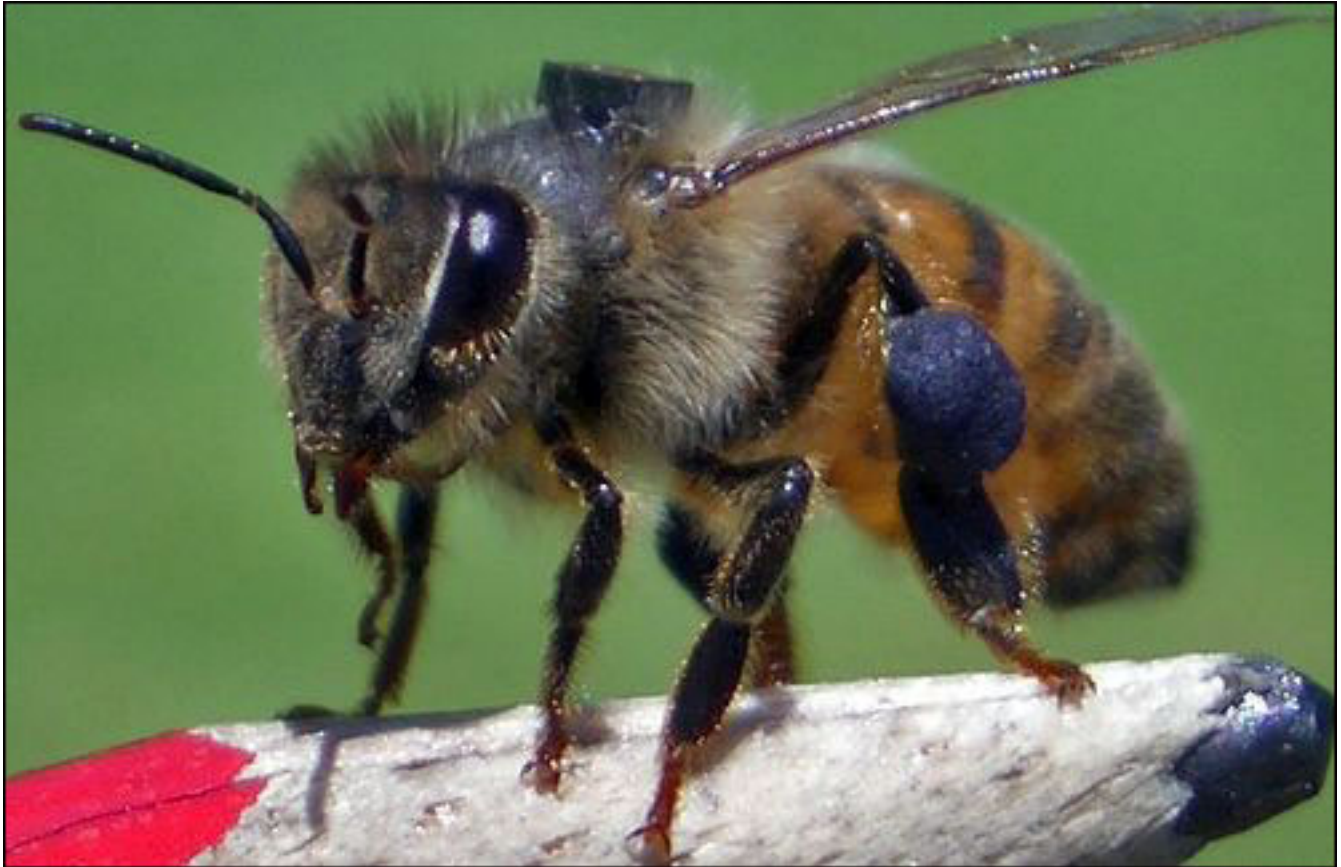
A passive 13.56 MHz RFID tag was glued to the back of each honeybee.
