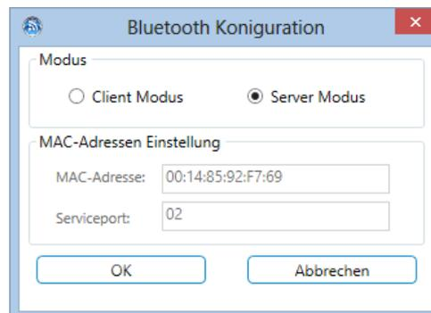
This dialog is used to set the Bluetooth-specific parameters. So you can switch between the operating modes "server mode" and "client mode" which are already mentioned.
