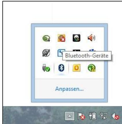
The COM port is the interface through which you can communicate with the POCKET from the software side in some cases, you need to know which COM port has been occupied by the POCKET. To find out which port has the POCKET occupied, select on the desktop "Bluetooth-device" and in the context menu "Open settings".
