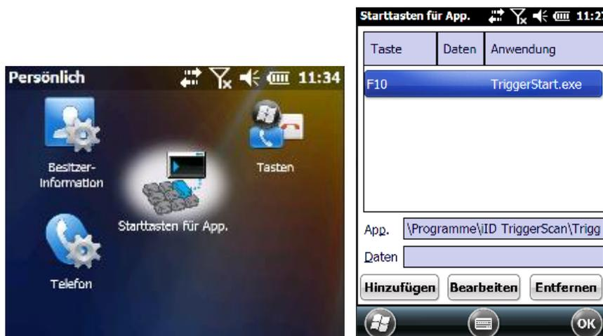
Ready: Pressing trigger within any application will cause iID TriggerScan to start and place scanned data into an input field.
